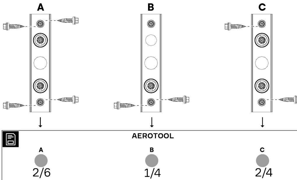
**i** The required number of screws for fixing the TR15 bracket is specified in the planning documents. The **first digit** indicates the quantity of drilling screws and the **second digit** indicates the number of thin sheet screws (lateral and vertical).
