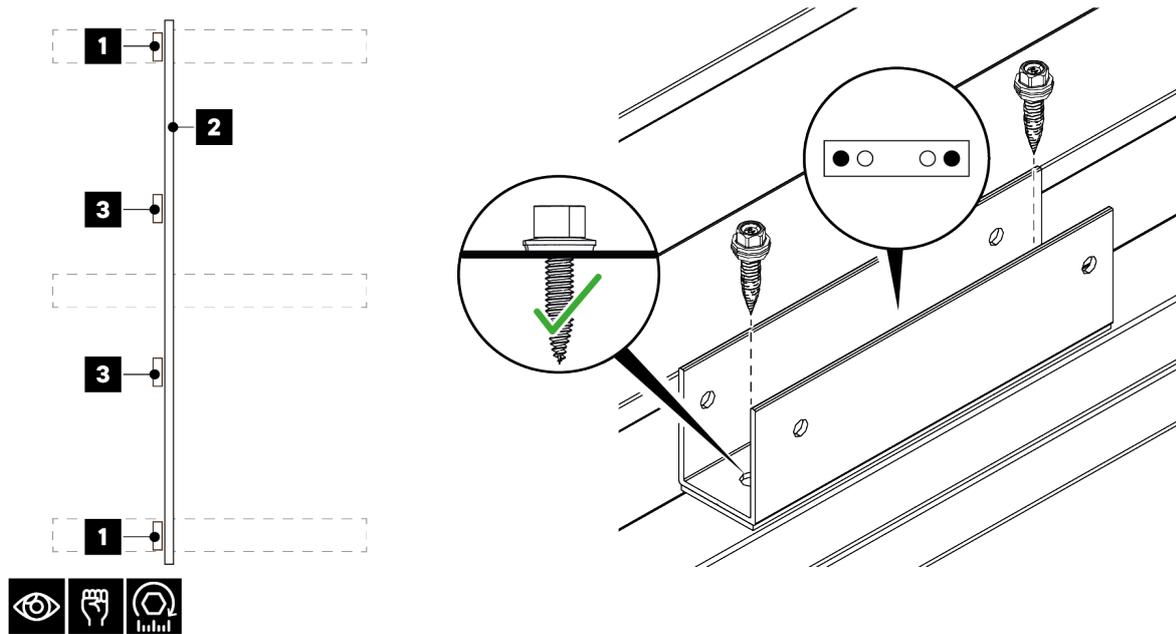
**i** It should be noted that the TR15 bracket are mounted in parallel. A mounting rail (2) serves as a useful aid here to facilitate mounting and ensure alignment.
