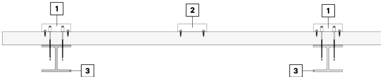
**i** The TR15 bracket (1), which are located in the area of the substructure (3), are fastened to the sandwich roof with thin sheet metal screws and to the substructure (3) with **additional drilling screws**. The TR15 bracket (2) in between serve as intermediate bearings and are only attached to the sandwich roof.
