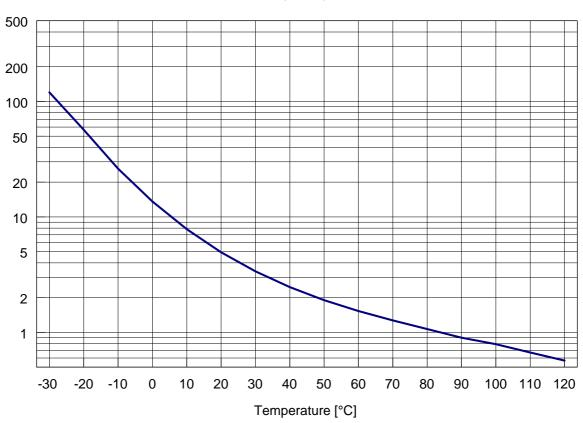
Kinematic Viscosity of Tyfocor<sup>®</sup> LS [mm<sup>2</sup>/s]
