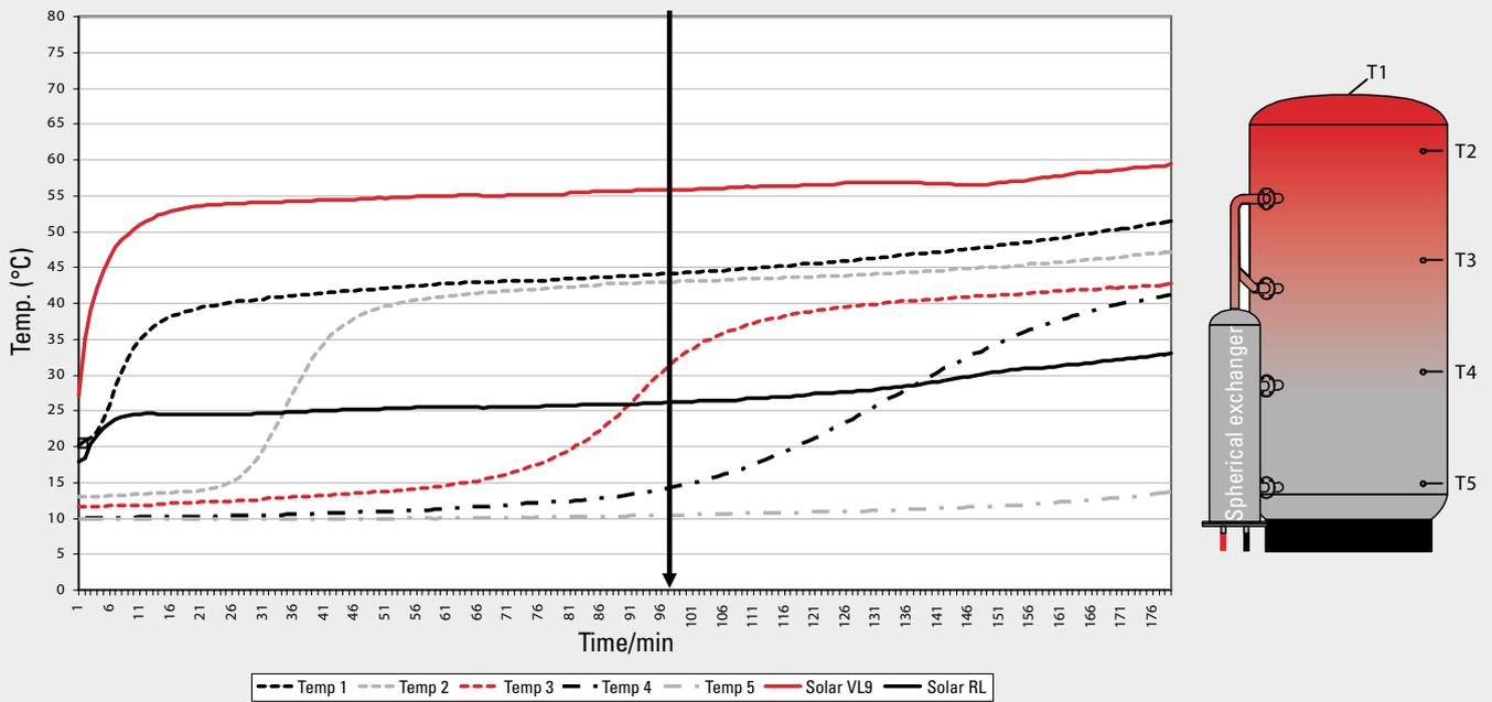
Data while heating using a spherical exchanger (ST20) with a flow volume of 400 l/h and a collector surface area of 16 m<sup>2</sup>. 13 kWh are required to obtain usable hot water at 40 °C (achieved within 98 min).
