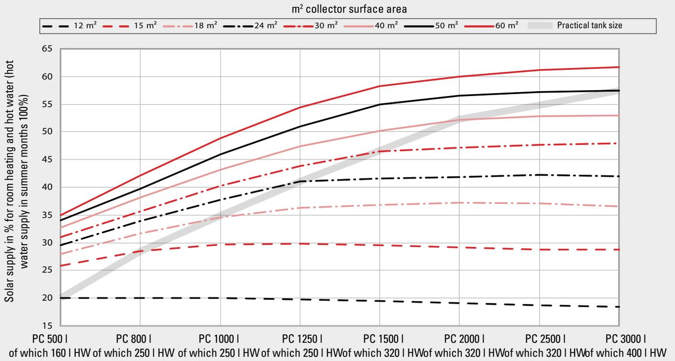
Reference house: 9 kW heat load at -15 °C ambient temperature
