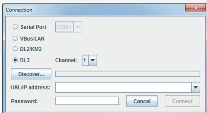
If you use a DL3, select the right channel for the controller you wish to access. Channel 1 is VBus<sup>®</sup> input 1 on the DL3, channel 2 is VBus<sup>®</sup> input 2 and so on.
