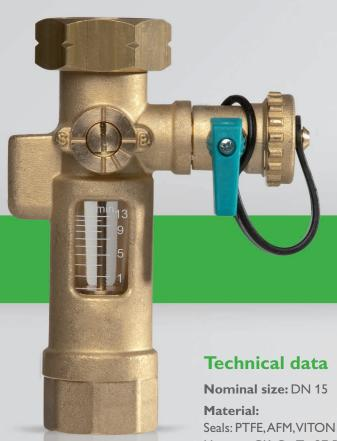
For the correct function of a solar thermal system, the right flow rate is important. The RESOLVM1020 flowmeter reliably indicates flow rates between 1 and 13 litres per minute, if necessary, the value can be limited by means of the integrated flow rate limiter. By means of the additionally integrated fill/drain valve, the system can be flushed and drained, for measuring the return temperature there is an opening for an immersion sensor.
